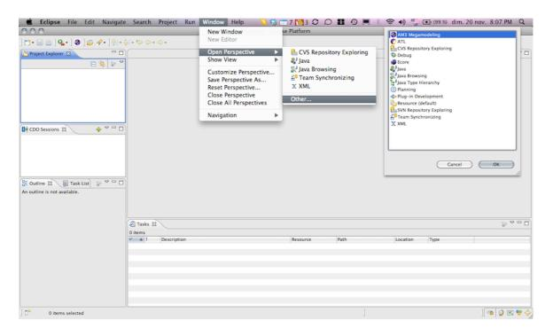
Create any model element in the megamodel left clicking in any element in the left panel, selecting new [element]. Give any value to the element and then use File->Save option to save the Megamodel. With this operation the Megamodel file is created in the filesystem.
