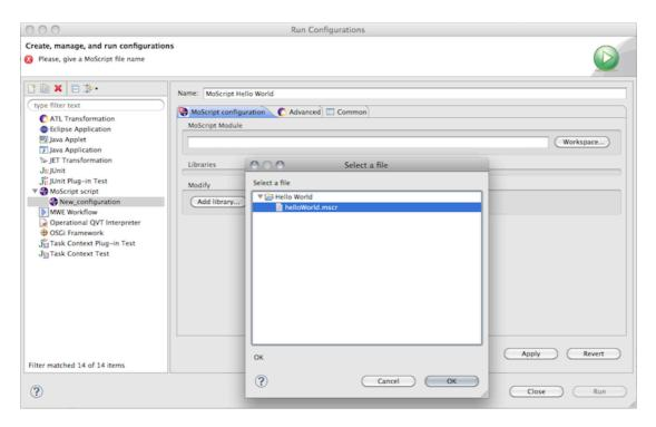
Browse in the workspace for the HelloWorld.mscr file and select it. Then, in the advanced tab, check the options Clear console before launch and Print execution times to console, so that you can clearly see when de script finishes.
